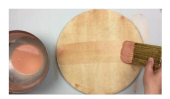
Let that settle in so it's not just so sopping wet. It doesn't need to be very dry. Then brush another coat on, this time working in the opposite direction. Each coat will help to even out the fine brush marks made in the previous layer.
