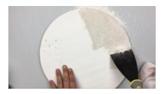
Keep scraping until the shelf is free from kiln wash. Give the shelf a wipe with a dry cloth. You'll have kiln wash scrapings all over your table now. You can use a HEPA filtered vacuum cleaner to clear them away or use a damp cloth. Keep your mask on when doing this.
