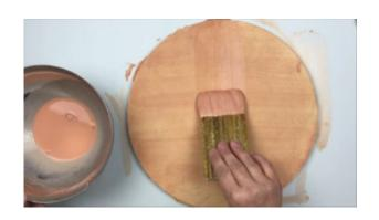
Finally add a fifth layer of kiln wash. No kiln shelf should be visible through the kiln wash. If it looks a bit patchy, you can add a few more layers.
